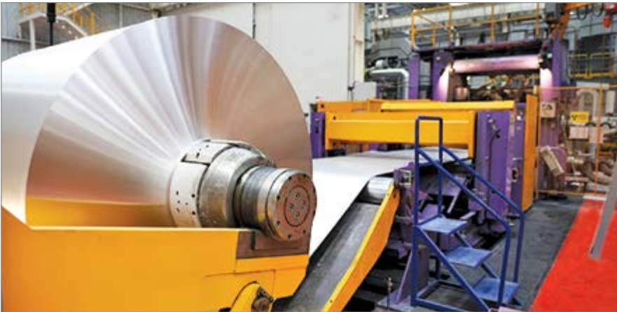
Deflector rolls ensure accurate foil alignment, maintain proper tension and guide the aluminum strip smoothly before final coiling.
