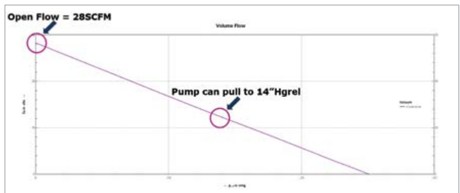
Figure 1. This graph illustrates the performance of a vacuum pump, showing that as vacuum level increases (lower pressure), the volume flow rate decreases.
