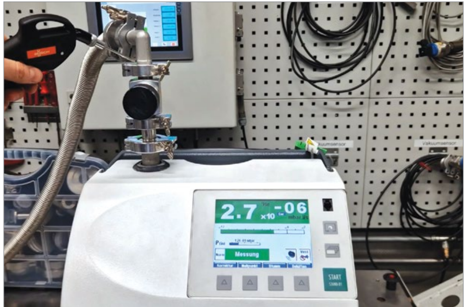
Perform leak tests in a clean environment with a stable temperature.
