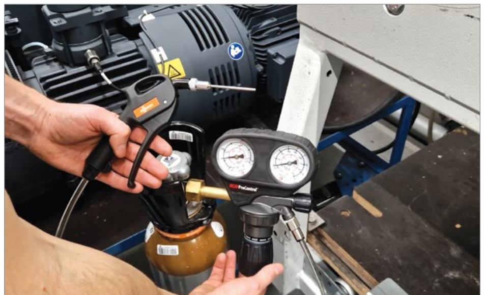
Perform calibrations regularly to preserve the accuracy of leak detection equipment.
